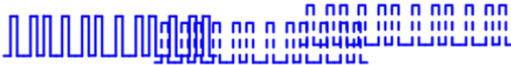
Fig. 2-4. A high bit rate signal in multipath fading channel.
